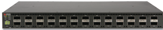
Figure 3: The Ruckus ICX 7750-26Q features 26 40 GbE QSFP+ ports that can be split into as many as 96 10 GbE SFP+ ports.
